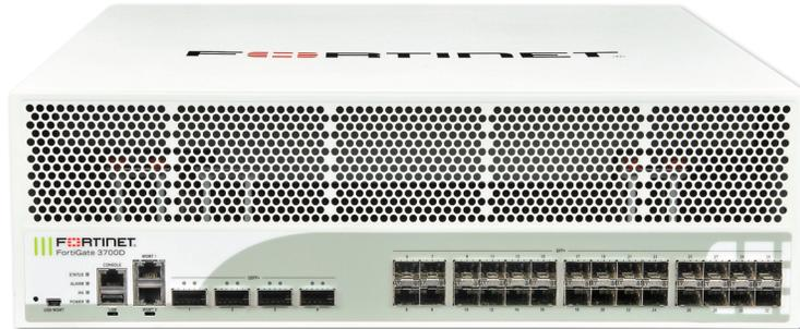
The FortiGate 3700D series delivers high performance threat protection and SSL inspection for large enterprises and service providers, with the flexibility to be deployed at the enterprise/cloud edge, in the data center core or internal segments. The multiple high-speed interfaces, high port density, superior security efficacy and high throughput of the 3700D series keeps your network connected and secure.
