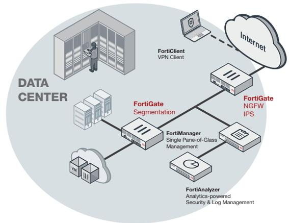
FortiGate 3700D deployment in data center (IPS/NGFW, Intent-based Segmentation)
