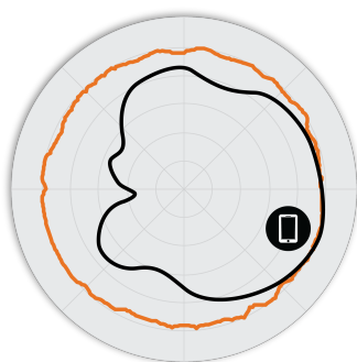
Figure 3. M510 5GHz Azimuth Antenna Patterns
