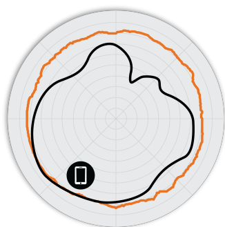
Figure 2. M510 2.4GHz Azimuth Antenna Patterns
