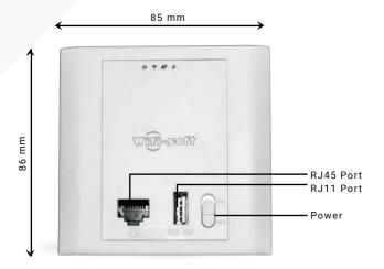
The diagram on the right shows the front panel of the access point. The AP comes with RJ-11 (PSTN phone) and RJ-45 port. These can be used for connecting laptop/switch for Internet access and regular phone.
